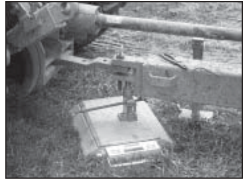
Figure 2. A jack placed on the load cell supports the weight of the spreader.
