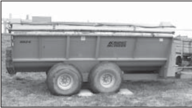
Figure 1. Load cells placed in front of manure spreader tires.
